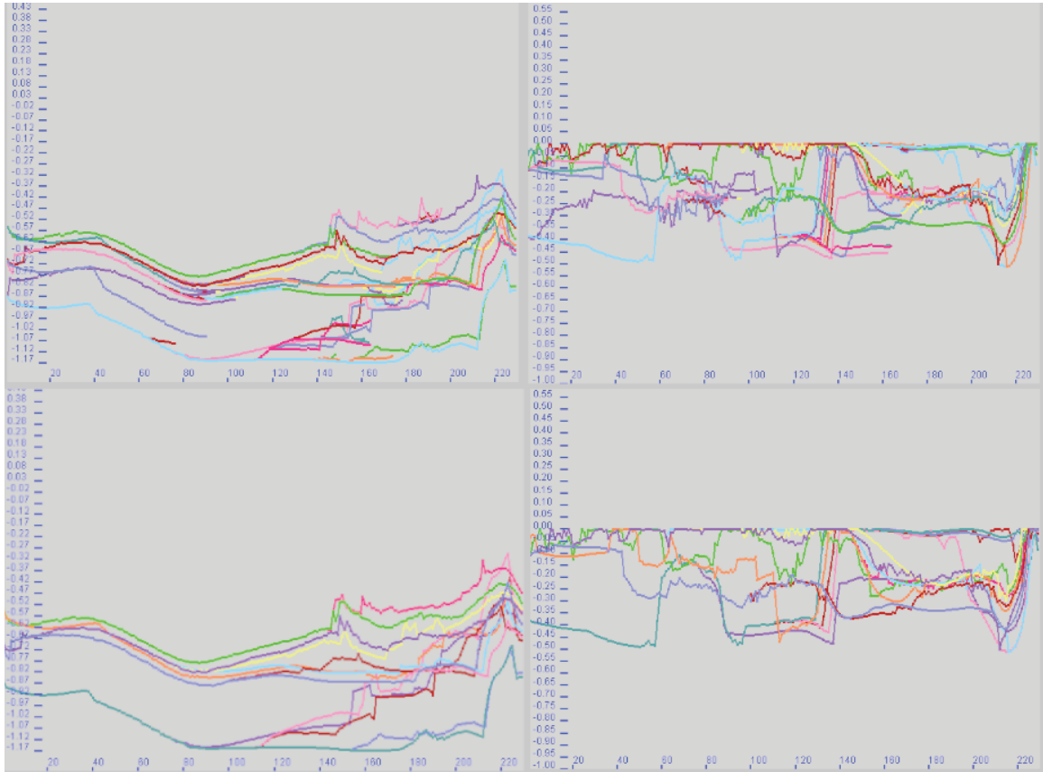
Figure 28: Search tree for a joint with 3000 nodes. Top left: z-axis of the MCP joint of the index finger; top right: z-axis of the PIP joint of the ring finger; bottom left: successful trajectories of the index finger; bottom right: successful trajectories of the ring finger.
