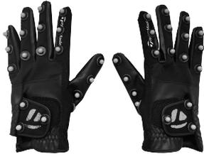
Fig. 2. **Dense marker set layouts.** We attach 19 adhesive reflective markers on each off-the-shelf golf glove. Three markers are placed at the back of the glove, and a marker is attached to the center of each finger bone segment. We build five pairs of gloves of different sizes to capture the full range of adult hand sizes. These gloves are easy to put on and remove, which streamlines capture preparation.
